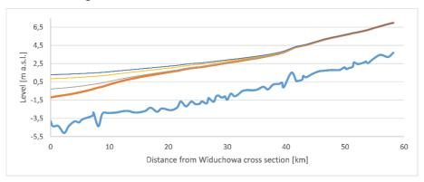
Fig. 4. Backwater curves for SSQ flows. Light blue – river bottom; orange – normal depth (without damming); grey - curve for  $Q = 599 \text{ m}^3/\text{s}$  and W = -0.275 m. a.s.l.; gold - curve for  $Q = 599 \text{ m}^3/\text{s}$  and W = 0.855 m. a.s.l.; blue - curve for  $Q = 599 \text{ m}^3/\text{s}$  and W = 1.292 m. a.s.l.
