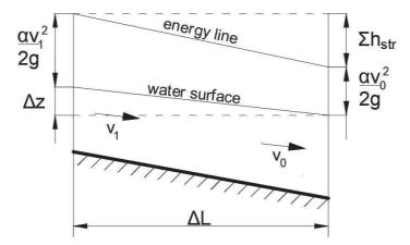
Fig. 1. The section of river contained between two cross-sections [3]
